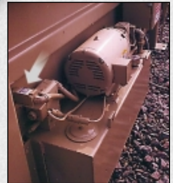
The RJ-225VL's Side-Mounted Power Unit shown without weather cover. Note the Limit Switch is also on the exterior of the compactor body.
