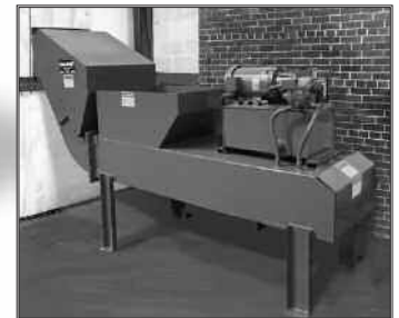
The RJ-30 is perfect for through-the-wall installations. Here the unit is fed from inside a building and the densely compacted log of waste is discharged on the opposite side of the wall.
