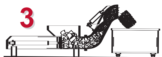
As waste enters the charge box, the ram pushes the forming log to the top of the "S" tube. This forces it from a vertical direction back to horizontal to form a continuous log throughout the "S" tube. Eighteen to twenty-four inch logs of refuse are gravity fed into the container.
