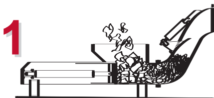
The packing ram forces materials from the charge box area into the patented "S" curve tube. Friction develops as it contacts the first part of the curve which starts the compaction process.
