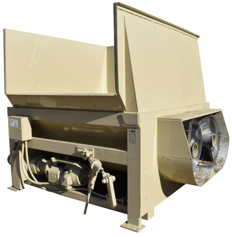
The AST-440 Stationary Auger Compactor is a heavy-duty machine specifically designed for compacting large volumes of waste material. As a Stationary Compactor, the machine is best suited for dry waste such as paper, cardboard, wooden pallets, etc. This Twin 28" Auger has excellent throughput. It's able to process large bulky items without bridging in the hopper and is commonly used for large industrial sites and production lines.
